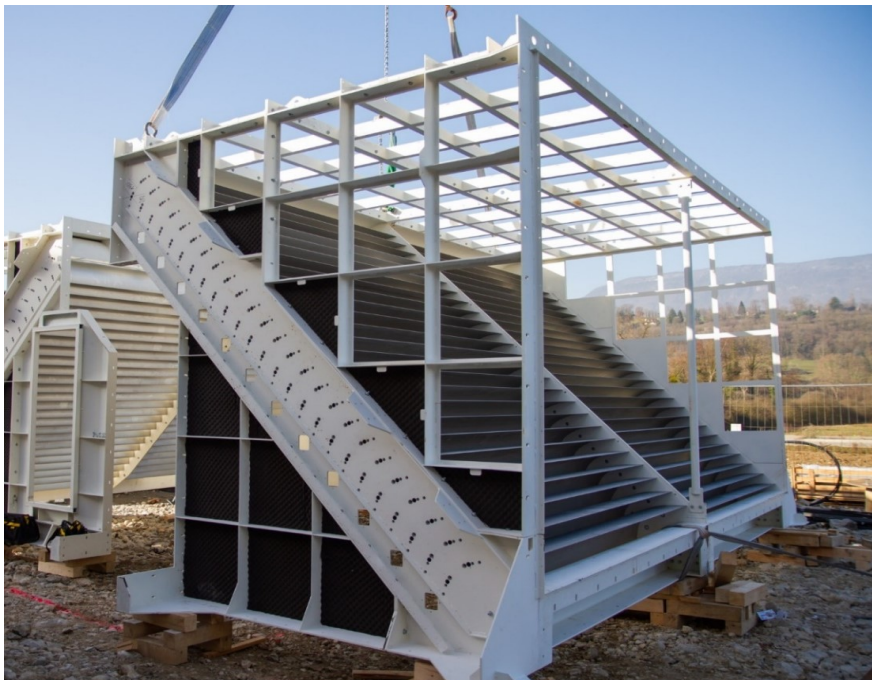
Fig. 2.4 2-component (double) TTE-TSA, air flow rotation downwards from the side. No cooling system manifolds are mounted.
